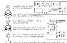
select "off" in order to disactivating the "instant trip function", by scrolling UP/DOWN buttons.
